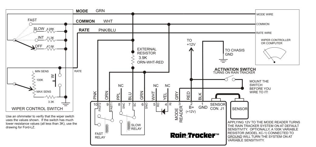
This drawing is for vehicles that DO NOT have depressed park. That is, when the wipers are off, they do NOT move to a lower position below the hood.
